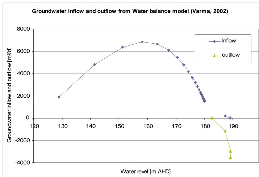
**Figure 27.** Groundwater inflow for Lake Kepwari (from Varma, 2002).
