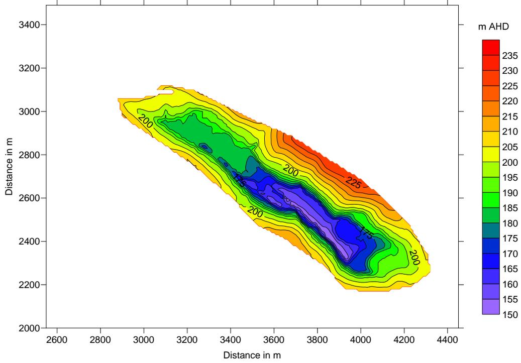
Figure 19. Bathymetry of Lake WO5C.
