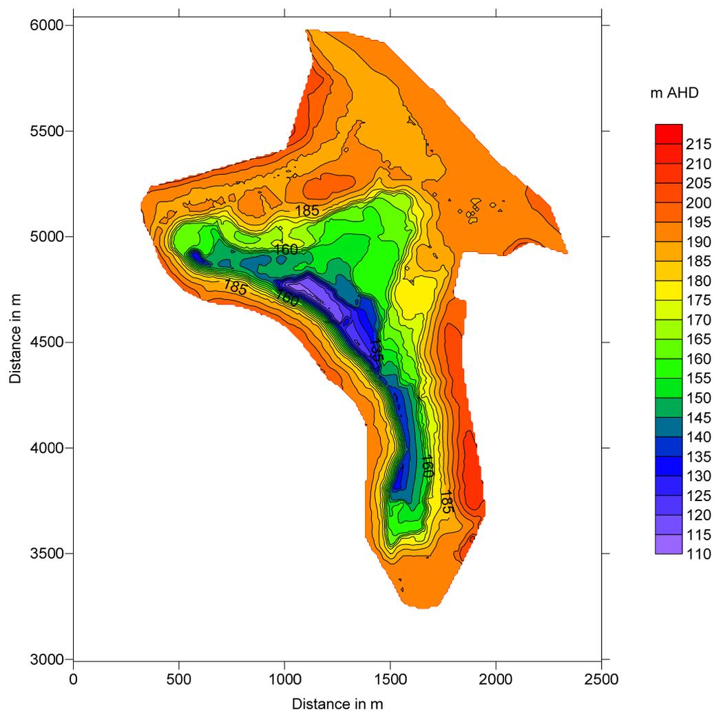
**Figure 14.** Bathymetry of Lake Kepwari.
