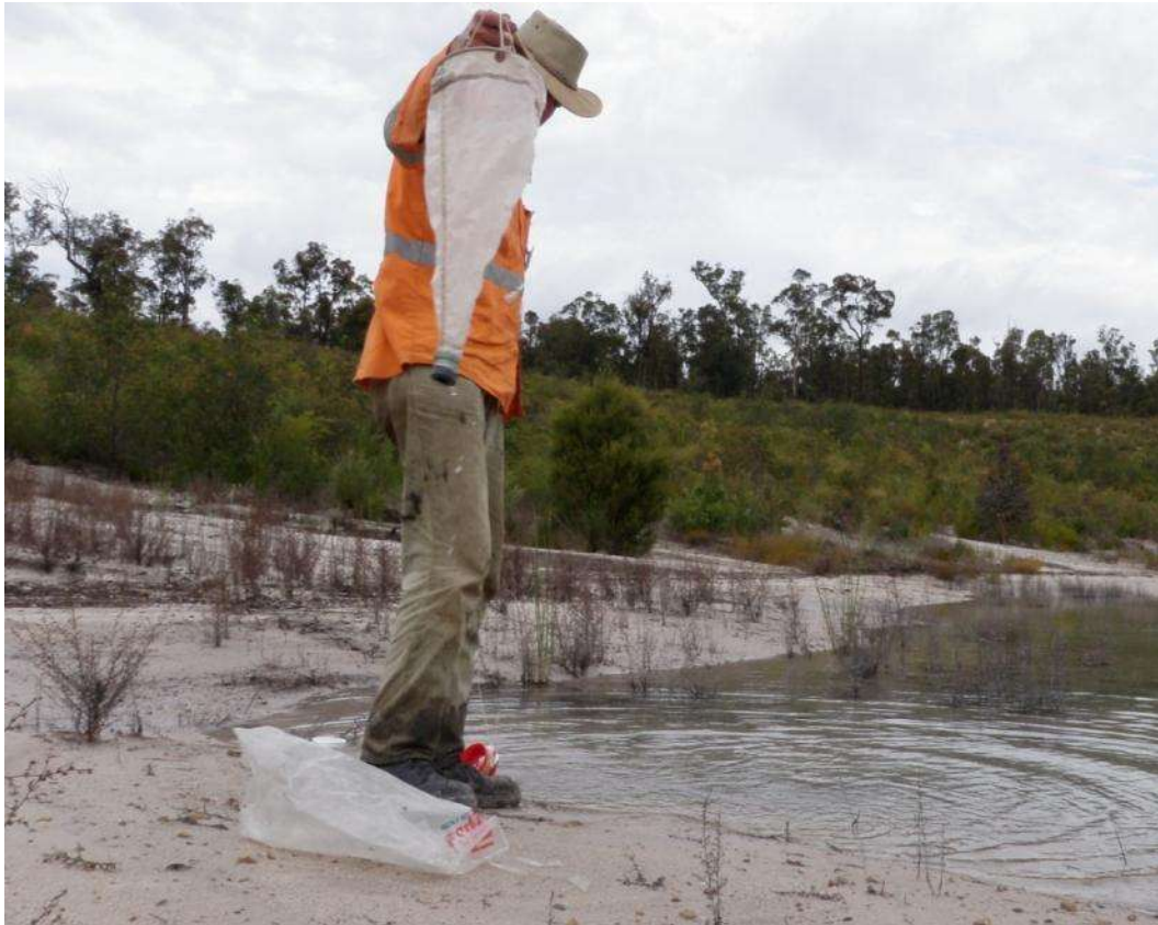
Plate 6. Where boat access is not available, a zooplankton net can be thrown and retrieved from shore as a horizontal tow instead.
