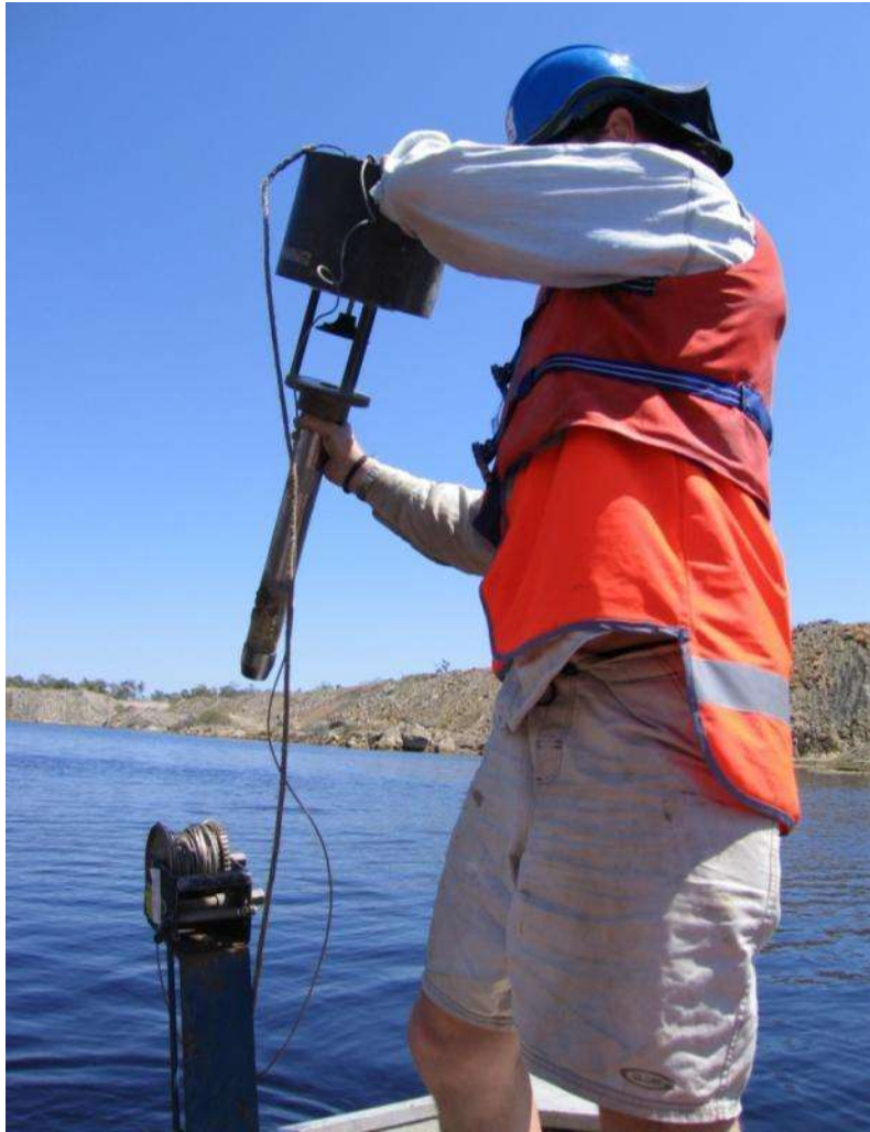
Plate 10. A “bomb” benthic sediment piston sampler being deployed into a pit lake from a small boat. Note winch to retrieve in left foreground.
