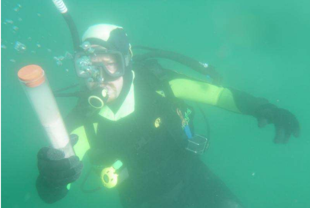
Plate 11. Divers can collect sediments from pit lakes using simple acrylic cores.
