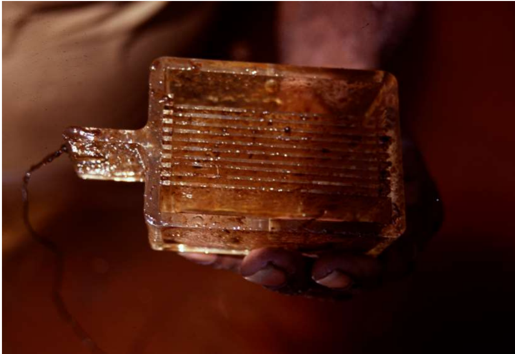
Plate 7. Artificial substrates, such as this glass slide-based ‘periphytometer’ allow easy quantification of periphyton abundances.
