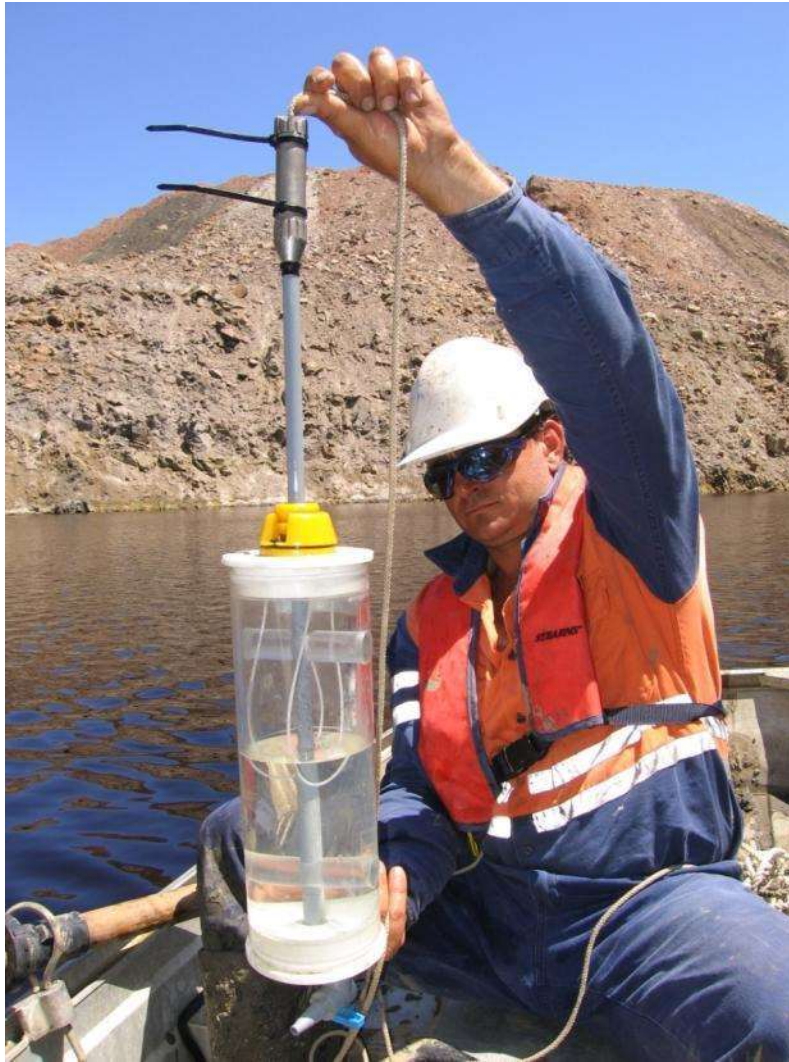
Plate 2. Kemmerer bottle sampling low redox hypolimnion waters of an acidic North Queensland pit lake.
